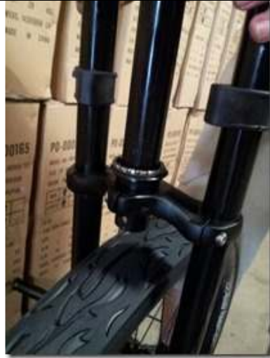
3) Insert O ring then Barring facing up on to fork
