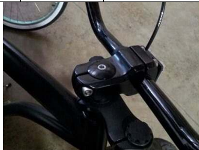
15) Insert stem and handle bar than insert the final cap with bolt tighten.
