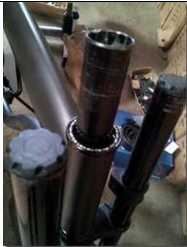
6) Insert on top of fork
