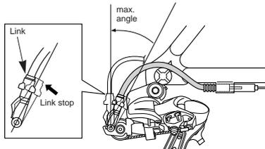
Connect the inner cable to the derailleur as shown in the illustration.
